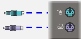
To use a PS/2 mouse or keyboard with your receiver or transmitter units, your system must be connected to the keyboard and mouse PS/2 connectors at the back of your transmitter unit and your keyboard and mouse connected to at least one of your units before your system and units are powered on.
